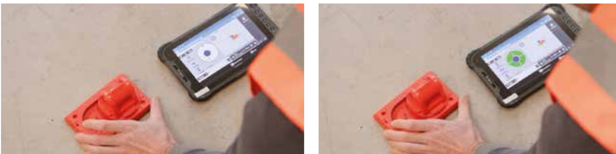
Move the stake out aid on the base plate until the target position is reached – visible on the green circle.
