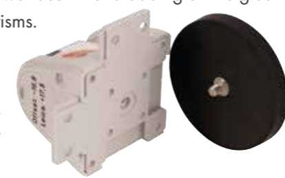
RSMP380 with Ø 25.4 mm mini prism: offset -16.9 (minus 16.9) [Leica +17.5] Tilting axis height RSMP380: 30 mm
