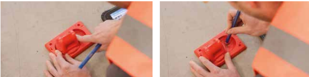
Slide the prism to one side and mark the target position with a pencil.
