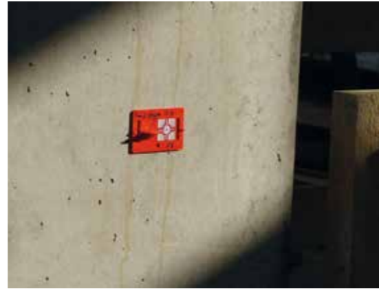
RS30r in industrial construction: a perfect measuring point for each measuring instrument.
